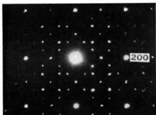
Fig. 1. (001) diffraction pattern of ordered \text{TiO}_{1.0} showing superposition of many orientations.
